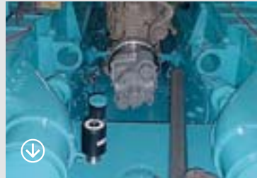
Hydraulic Drive on Amphibious Vehicle High pressure pump and motor installed below deck
