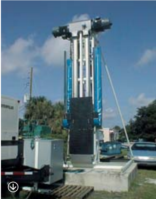
Acceleration Test Bed for NASA Acceleration testing at constant 4G's
